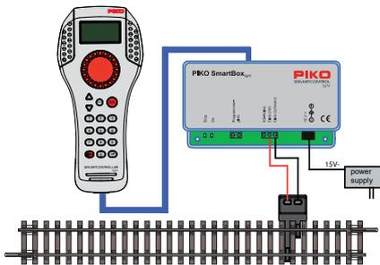
Next, turn on the operating voltage by plugging the power supply into the power outlet. A switchable multi-socket outlet can be beneficial.
