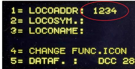
To make the selection of a loco easier, you can assign a symbol to each loco address (in our example the symbol of an ICE). To do that, please press [2] to reach the sub-menu 2 „LOCOSYM.“. Here, you can use the **up / down** ([▲] / [▼]) keys to select a suitable loco symbol. Confirm the symbol by pressing [↵].
