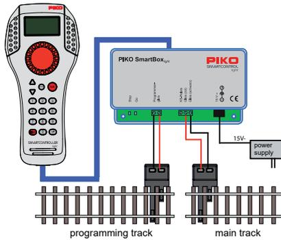
The programming track serves only for the programming of DCC decoders. During operation it carries no current and must not be connected to the main track.
