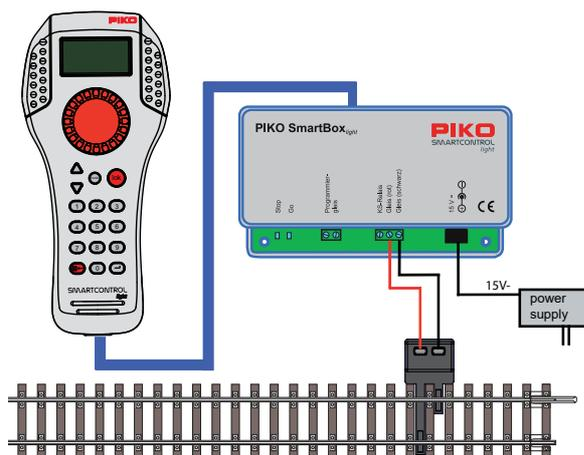
Connect the **PIKO SmartControl<sub>light</sub>** components according to the installation diagram and turn on the operation current by plugging in the power supply into the power socket. The green control LED will light up and the loco mode of the **PIKO SmartControl<sub>light</sub>** will be activated.
