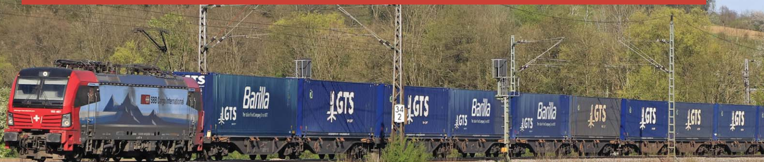
"Il treno della pasta". Carro bi-modulo da 90 piedi GTS con casse mobili "Barilla" e "GTS". "Pasta train". Container wagon Type Sggmrss '90 GTS with "Barilla" and "GTS" containers. "Der Nudel-zug. 90-Fuß-GTS-Bimodul-Wagen mit Barilla- und GTS-Wechselpritschen.
