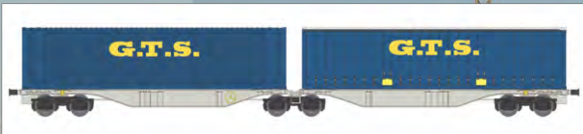
Carro intermodale Tipo Sggmrss '90 bimodulo noleggiato "GTS Rail" con carico di casse mobili. Container wagon Type Sggmrss '90 hired by "GTS Rail" with swap bodies. Containerwagen Typ Sggmrss '90 Doppelmodul vermietet an "GTS Rail" mit Wechselpritschen.
