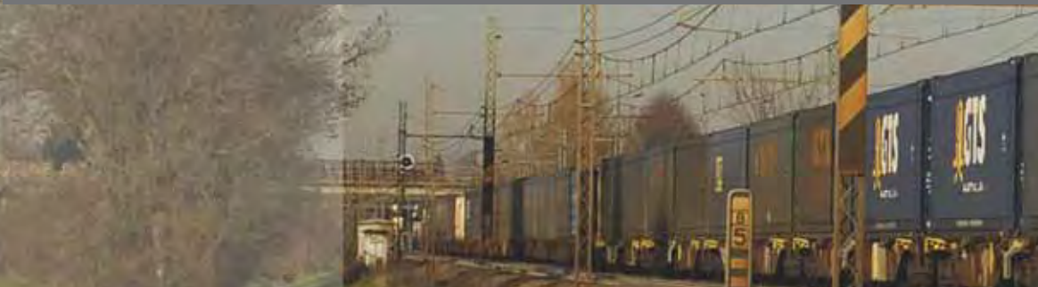
Carro intermodale Tipo Sggmrss '90 bimodulo noleggiato "GTS Rail" con carico di casse mobili. Container wagon Type Sggmrss '90 hired by "GTS Rail" with swap bodies. Containerwagen Typ Sggmrss '90 Doppelmodul vermietet an "GTS Rail" mit Wechselpritschen.
