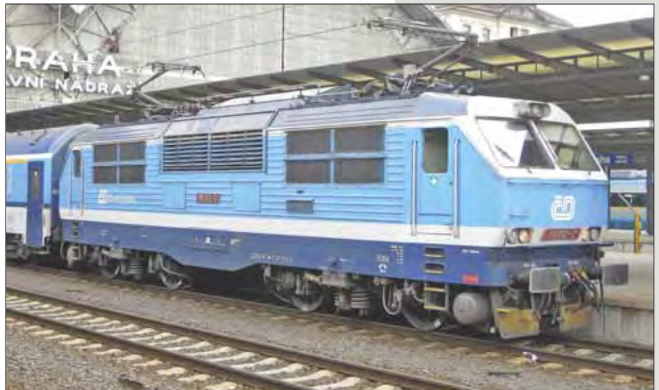
Locomotiva Classe 151 006 delle Ferrovie Ceche ČD per treni intercity. Class 151 006 locomotive of the ČD (Czech Railways) for intercity trains. E-Lok Baureihe 151 006 ČD (Tschechische Eisenbahnen) für Intercity-Züge.
