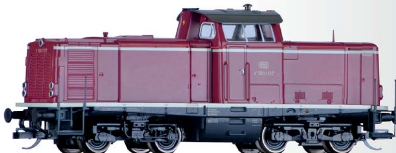
Diesellokomotive V100.10 der DB Diesel locomotive class 100.10 of the DB
